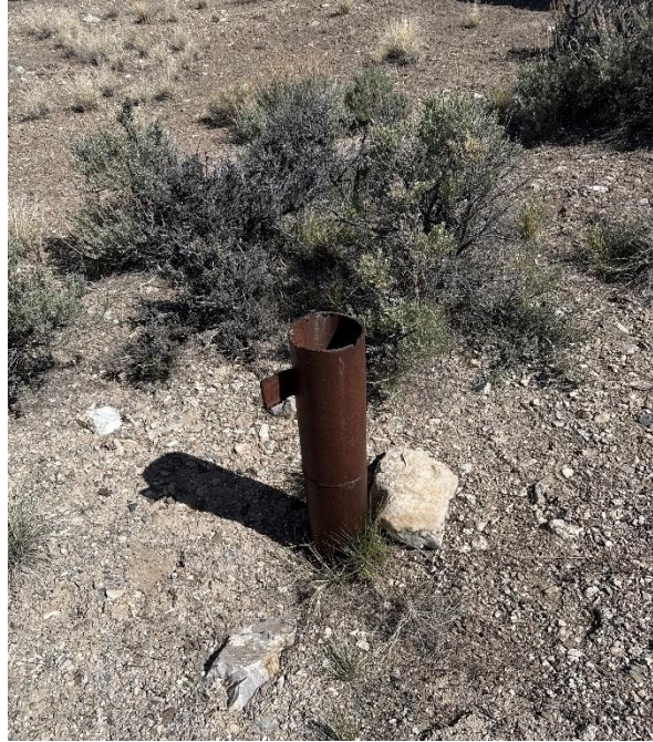
Figure 9.8. Historic drill collar.
